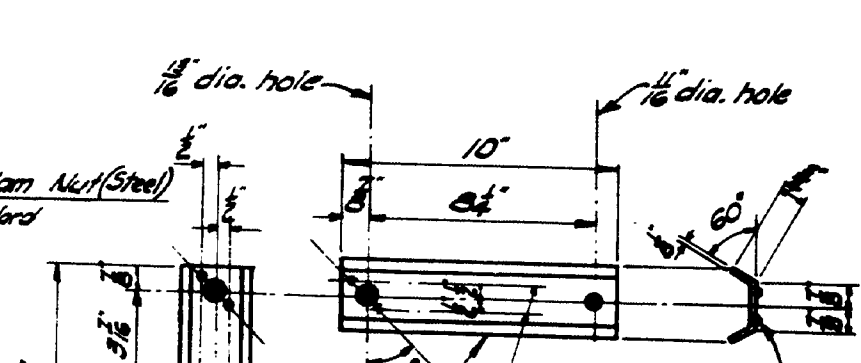
STEEL SPACERS FOR ANCHORAGE ASTM A 36
